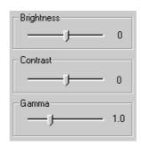
Dragging a slider to the left decreases the level and to the right increases it. The number at the right of each slider displays the brightness (value range: - 128 to +128, default: 0), contrast (-30 to 30, default: 0), or gamma value (0.2 to 3.0, default: 1.0).
